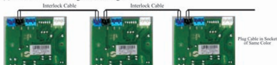
Figure 3-9 Network System Wiring with Interlock Cable
